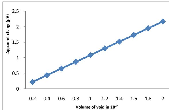
Fig 6: Variation of apparent charge for different volume of the void
