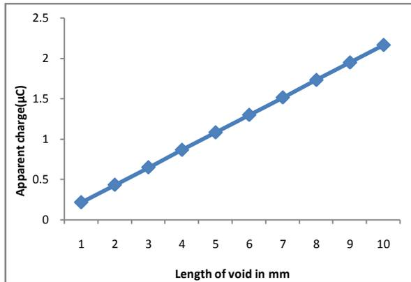
Fig 4: Variation of apparent charge for different length of the void, where b and t are constants (b=5mm and t=4mm).
