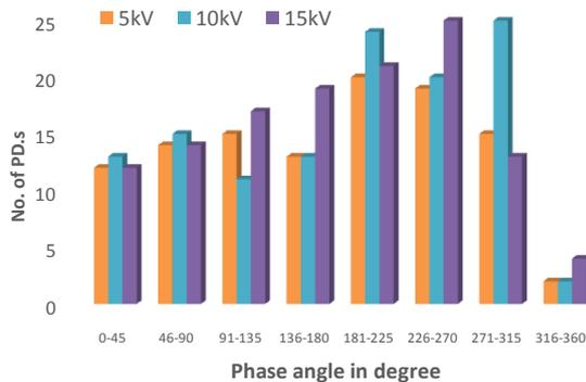
Fig 13: Partial discharge pulses at different phase angle with different applied voltages in cubical void.
