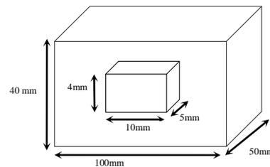
Fig 1: Void model of epoxy resin insulator with cubical void
